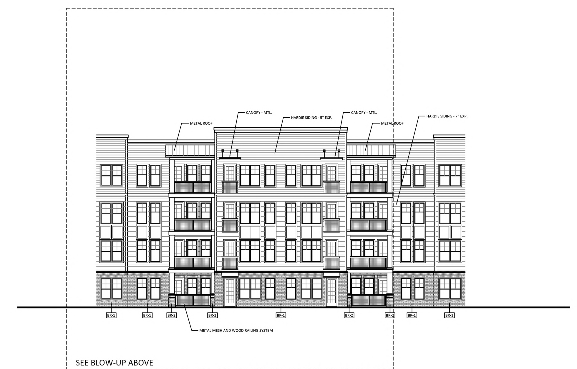
COURTYARD WEST EXTERIOR ELEVATION SCALE: 1/16" = 1'-0"
