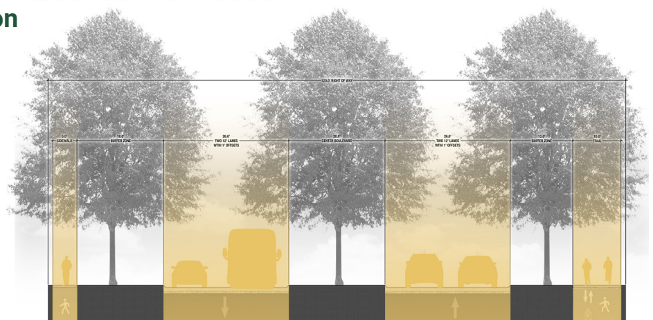
Minor Arterial Section
