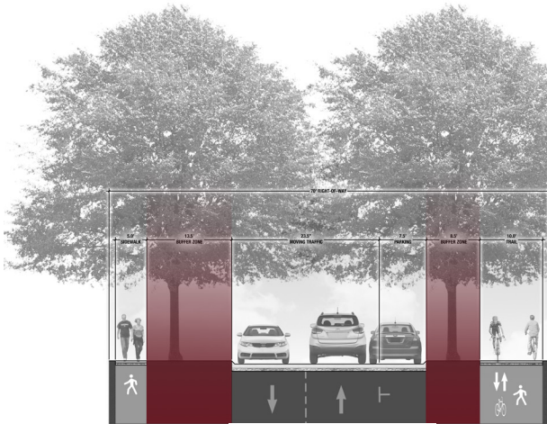
Minor Collector Section
