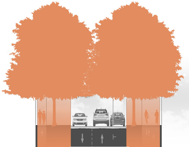
Minor Collector Section
