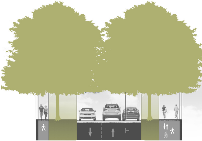
Minor Collector Section
