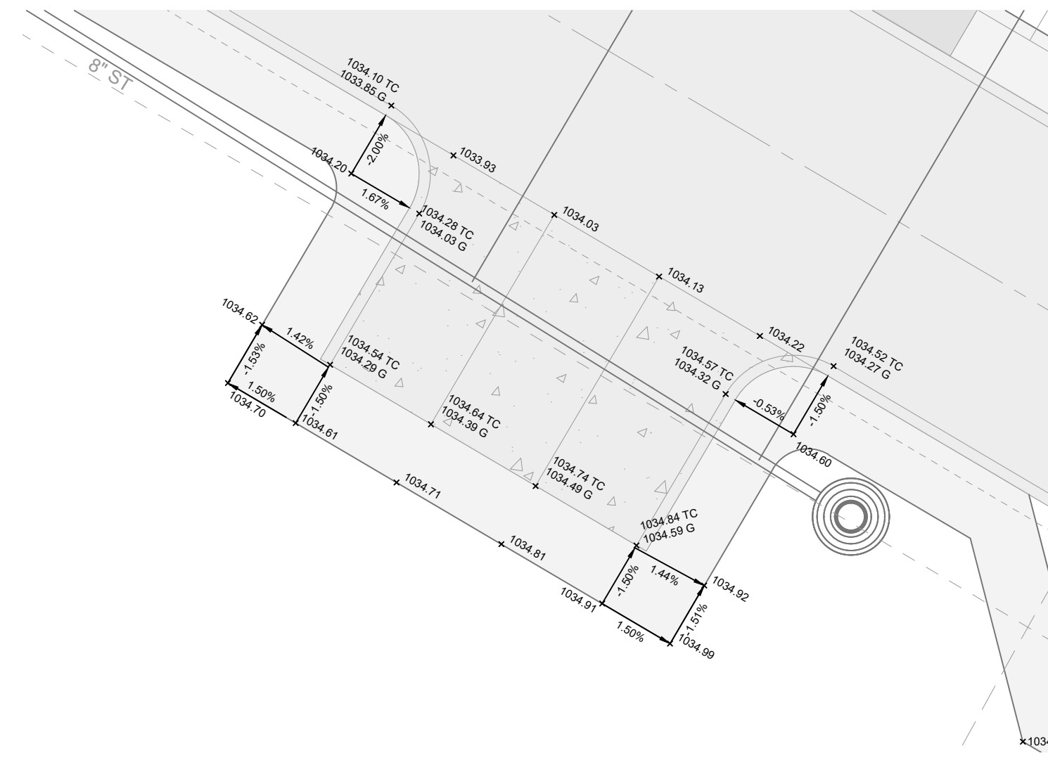
DETAIL N: PARKING DETAIL 1" = 10'
