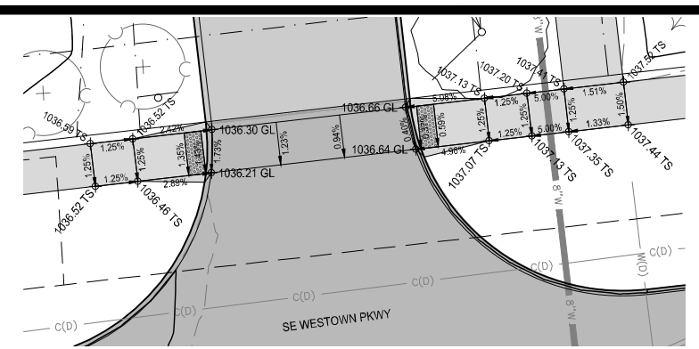
DETAIL A - ADA GRADING SCALE: 1" = 10"
