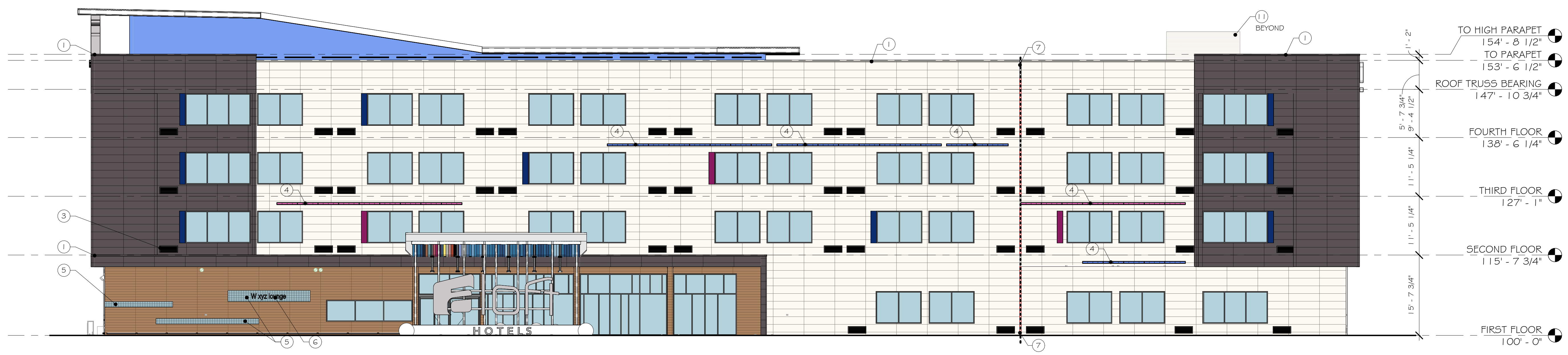
1 WEST EXTERIOR ELEVATION SCALE: 3/32" = 1'-0"
