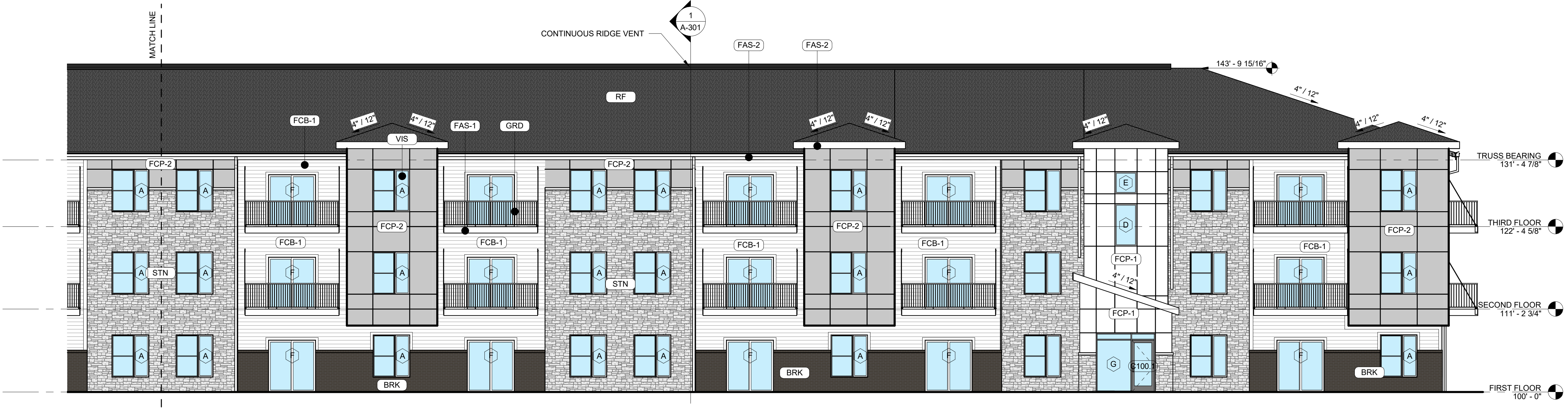
1 BLDG TYPE B - FRONT ELEVATION SCALE: 1/8" = 1'-0"
