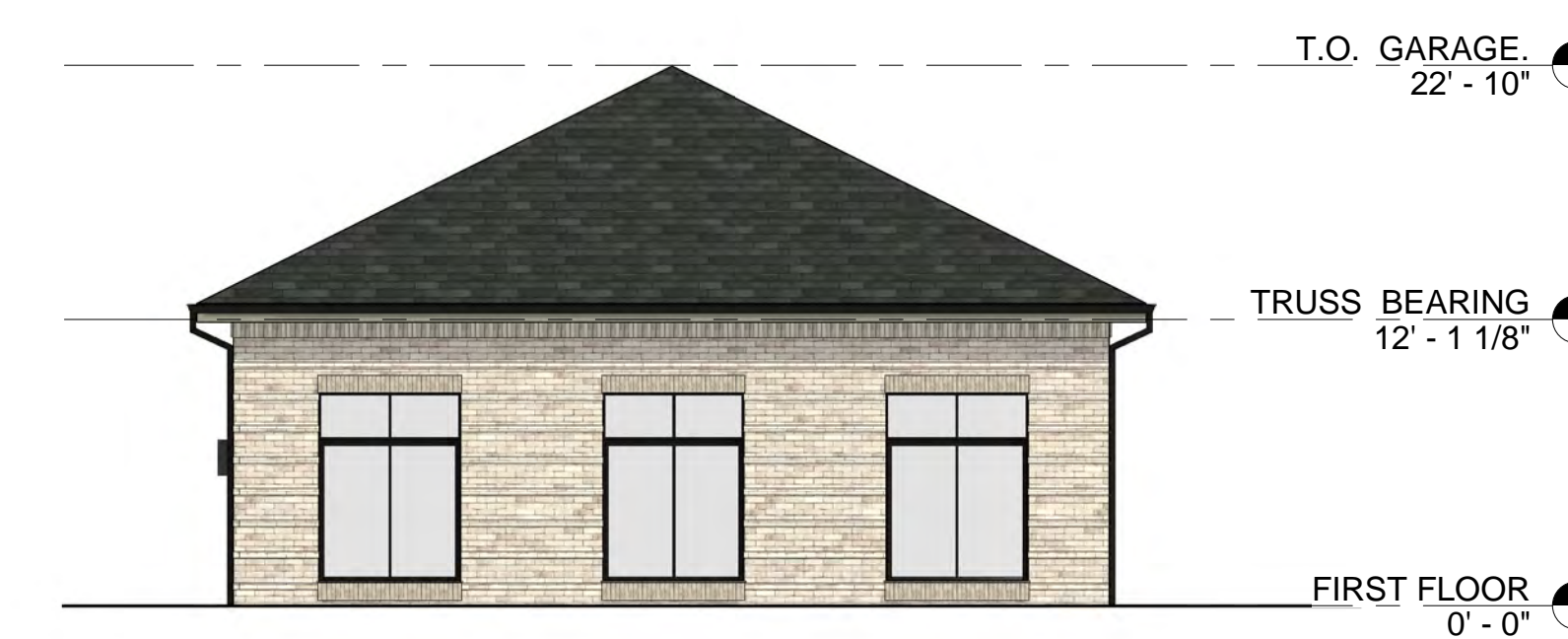
03 GARAGE B ELEVATION SOUTH 1/8" = 1'-0"
