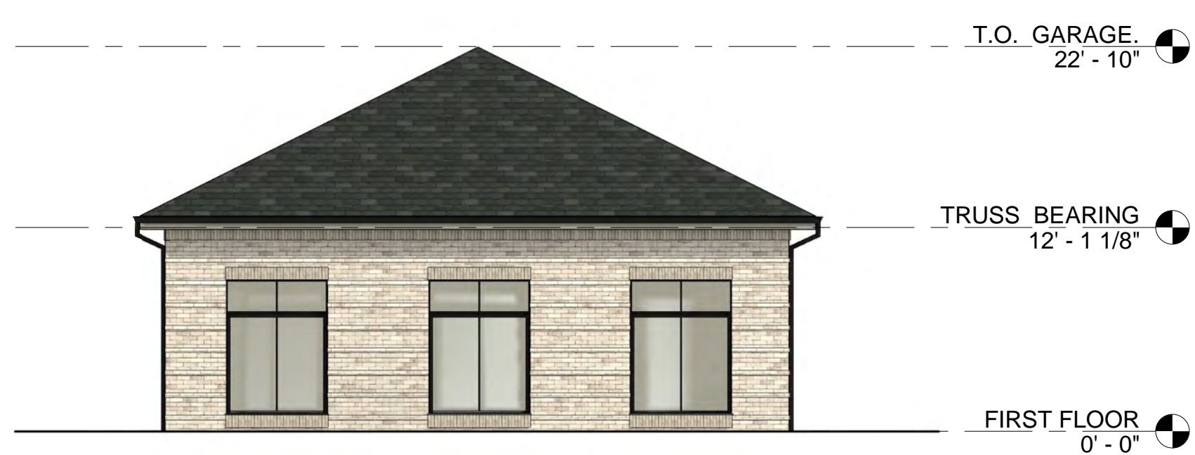
06 GARAGE A ELEVATION NORTH 1/8" = 1'-0"
