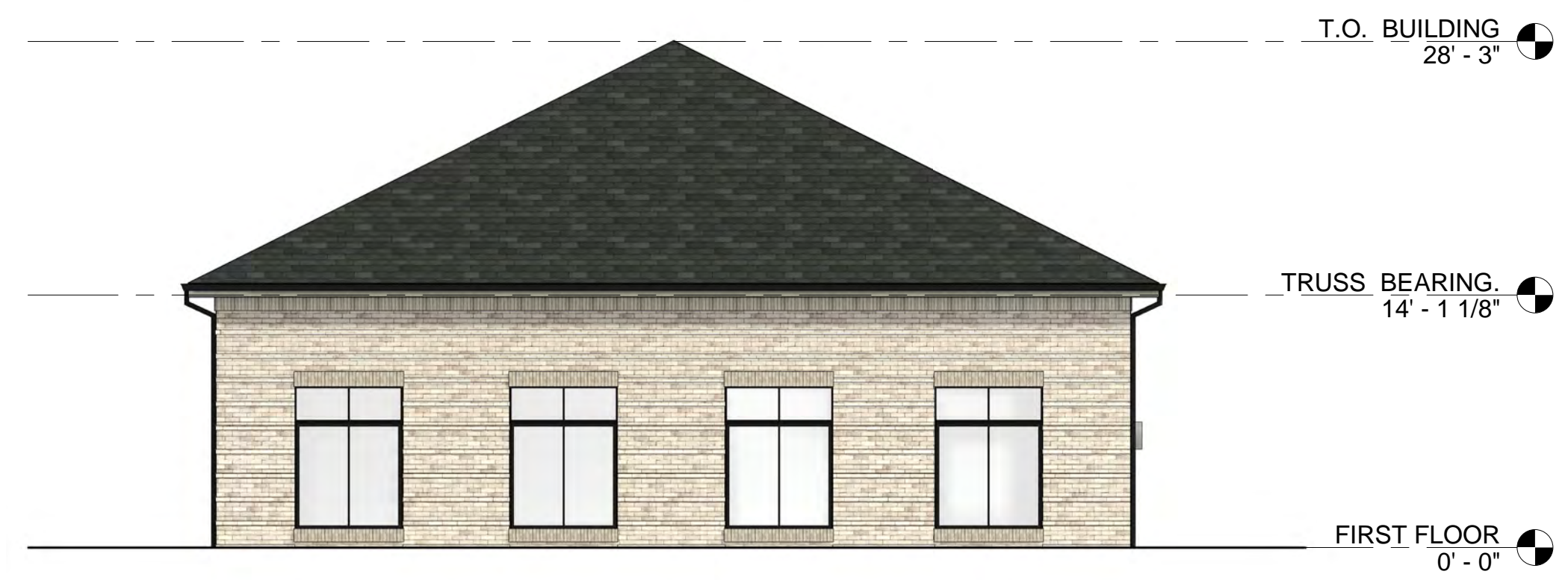
03 MAINTENANCE ELEVATION NORTH 1/8" = 1'-0"
