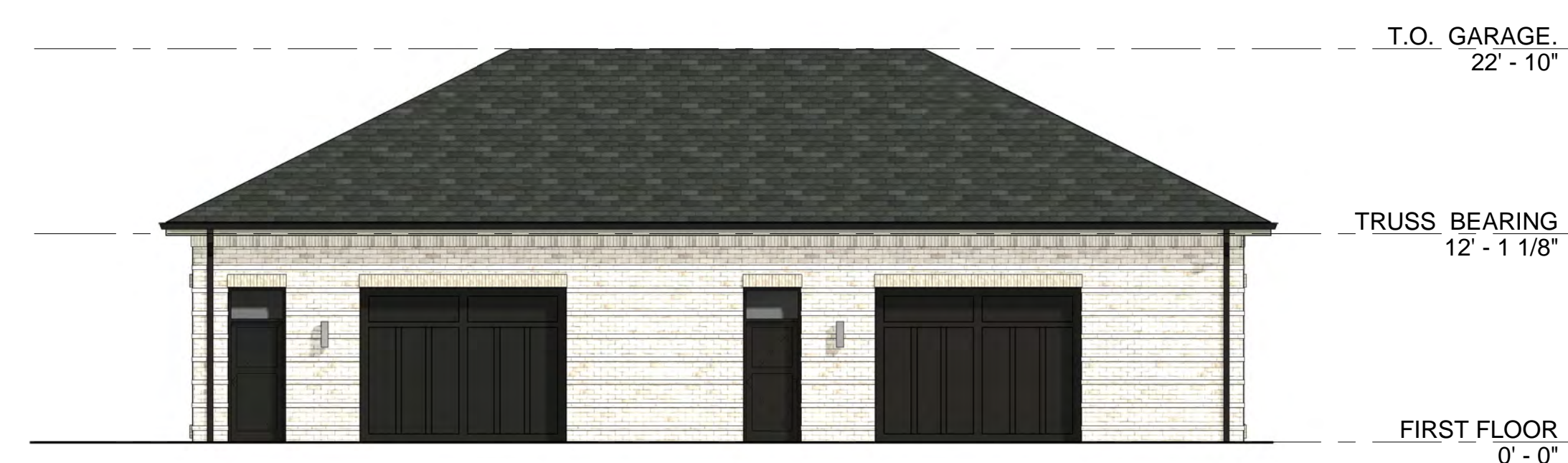
01 GARAGE B ELEVATION WEST 1/8" = 1'-0"
