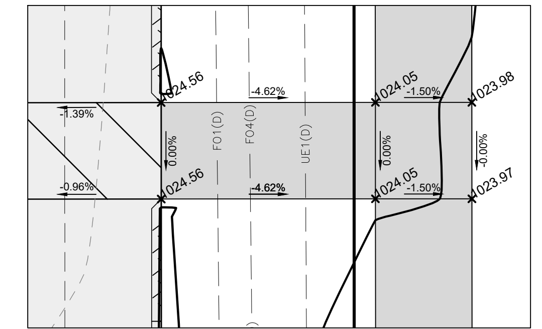
SOUTH SIDEWALK CONNECTION DETAIL SCALE: 1" = 5'
