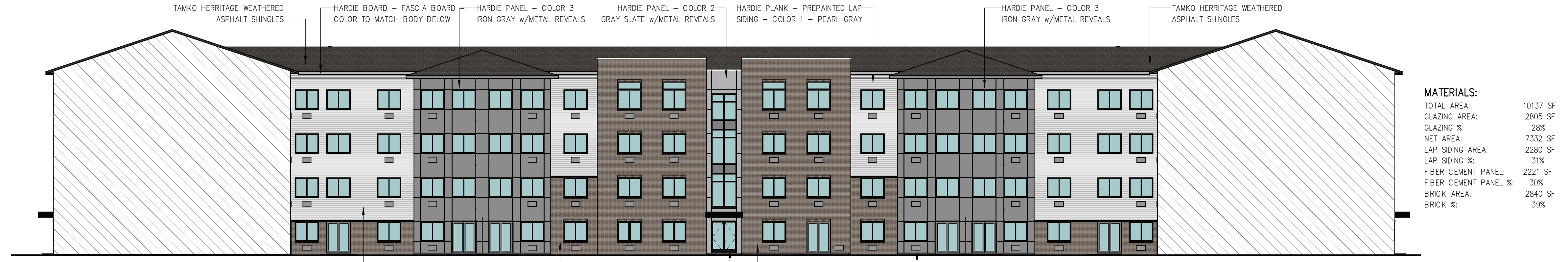
4 COURTYARD WEST ELEVATION 1/16" = 1'-0"
