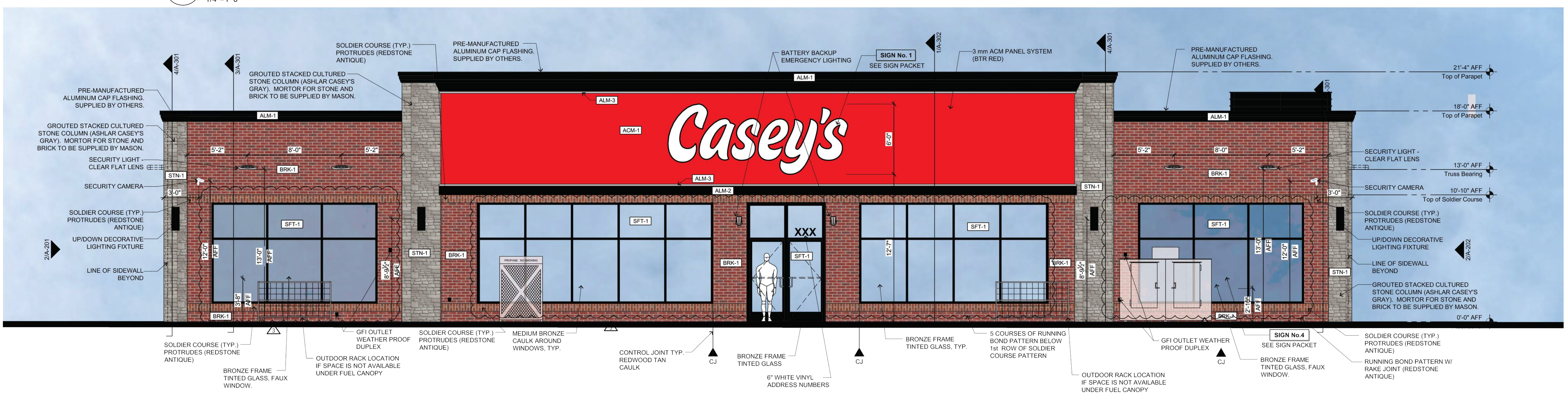
1 East Elevation - Front of Building 1/4"=1'-0"
