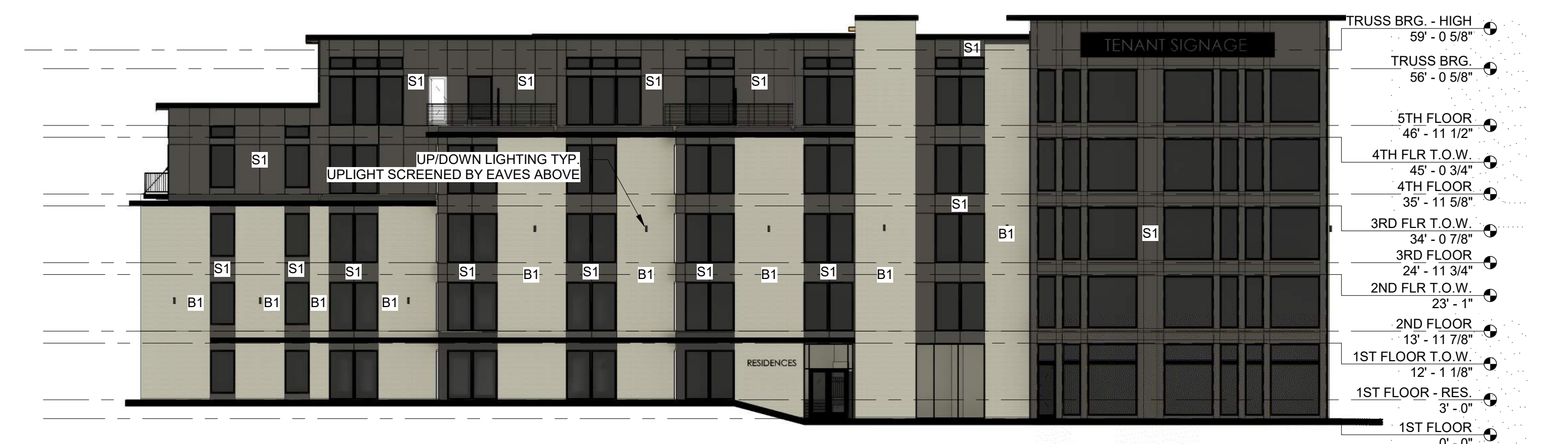
1 NORTH ELEVATION SCALE: 1/16" = 1'-0" 4,088 SF GLAZING 11,033 SF TOTAL 37% GLAZING 958 SF GLAZING (1ST FLOOR) 2,354 SF TOTAL (1ST FLOOR) 40.7% GLAZING
