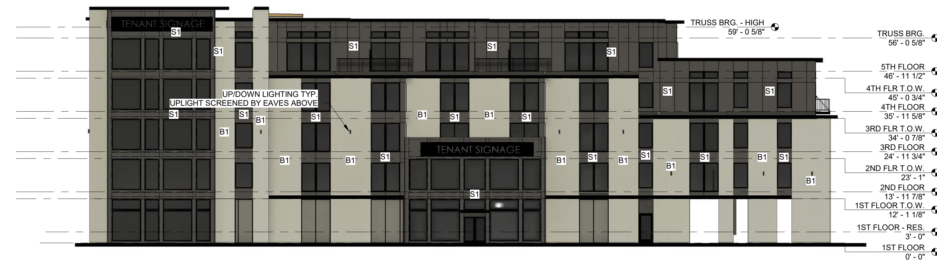
2 WEST ELEVATION SCALE: 1/16" = 1'-0" 4,169 SF GLAZING 11,684 SF TOTAL 35.7% GLAZING 1,058 SF GLAZING (1ST FLOOR) 2,262 SF TOTAL (1ST FLOOR) 46.8% GLAZING (1ST FLOOR)
