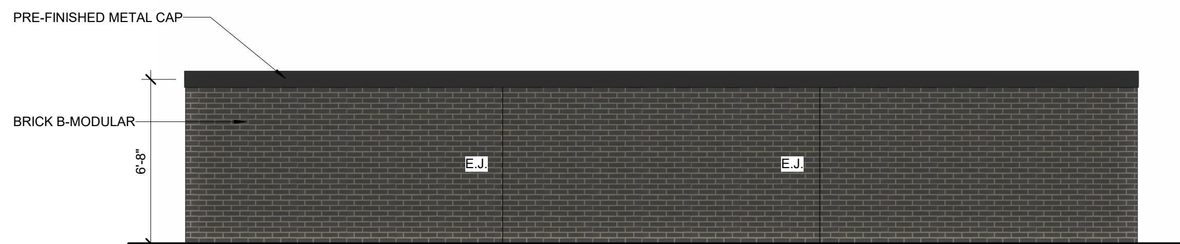
2 EXTERIOR ELEVATION - BACK OF TRASH ENCLOSURE 1/4" = 1'-0"
